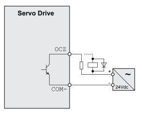
Inductive loads using DC voltages may damage the signal outputs. A protection circuit is required to protect the signal outputs against inductive loads.
