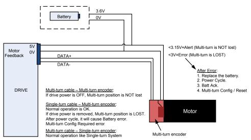
The multi-turn encoder is connected to the servo drive over a battery compartment, which is responsible to supply battery to the multi-turn subsystem in the encoder while power (5V) is off. The battery compartment contains circuitry which controls the switching between the power (5V) and the battery supply automatically.
