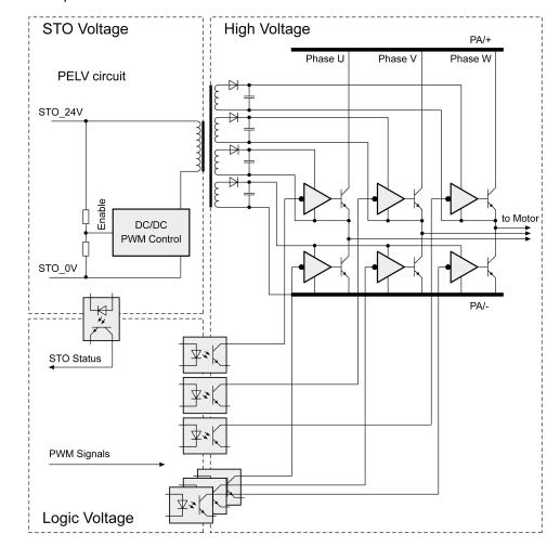
The safety function STO switches the supply voltage of the IGBT drivers so that PWM signals cannot switch the IGBTs. The following diagram illustrates the concept:
