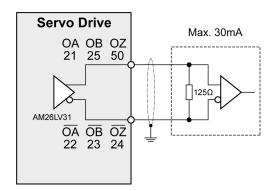
Example of encoder output signal, high-speed optocoupler.
