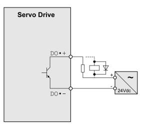
Example of digital output OCZ with internal power supply (negative logic):
