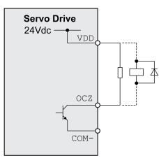
Example of digital output OCZ with external power supply (negative logic):
