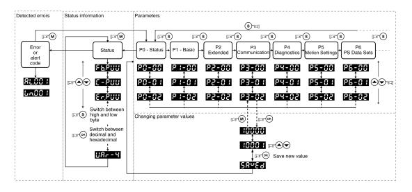
When the drive is powered on, the display shows the name of the selected status information function for approximately one second; after that, it displays the corresponding actual value or status value.
