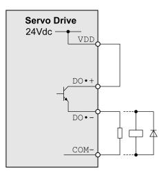
Example of digital outputs DO1 ... DO4 with external power supply (positive logic):
