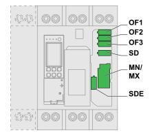
The electrical auxiliaries OF1, OF2, OF3, SD, and SDE can be:
