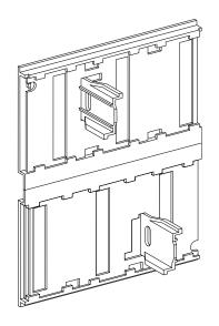
Top shutter locked. Bottom shutter not locked.
