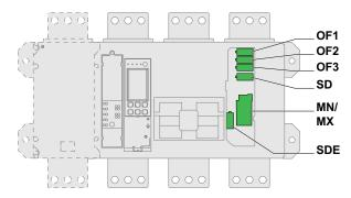
The electrical auxiliaries OF1, OF2, OF3, SD, and SDE can be:
