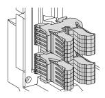
The sliding connections between the chassis and device are made up of two parts: clusters and disconnecting contacts. Grease between the clusters and the disconnecting contacts facilitates the connection and avoids damaging the silver-coated surface by reducing the racking-in friction.
