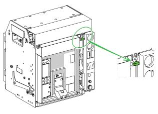
When the door is open, the racking handle cannot be inserted.
