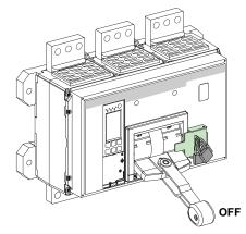
NOTE: The circuit breaker trips even when locked in the ON position.
