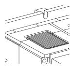
During a short-circuit, the arc chute extinguishes the arc and absorbs the high level of energy along the entire path of the short-circuit. Arc chutes also help to extinguish arcs under rated current conditions.
