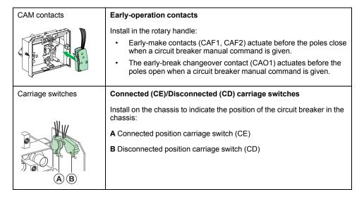
Operation of connected/disconnected carriage switches
