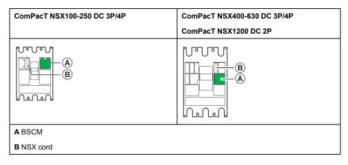
The BSCM cannot be installed at the same time as an OF contact or the SDE contact.
