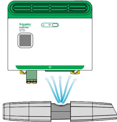
6. Slide the tester cap to close the tester and stop the spray.
