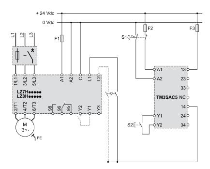
**S1** Emergency stop button with two NC contacts, Harmony XB4 or safety limit switches Preventa XCS.
