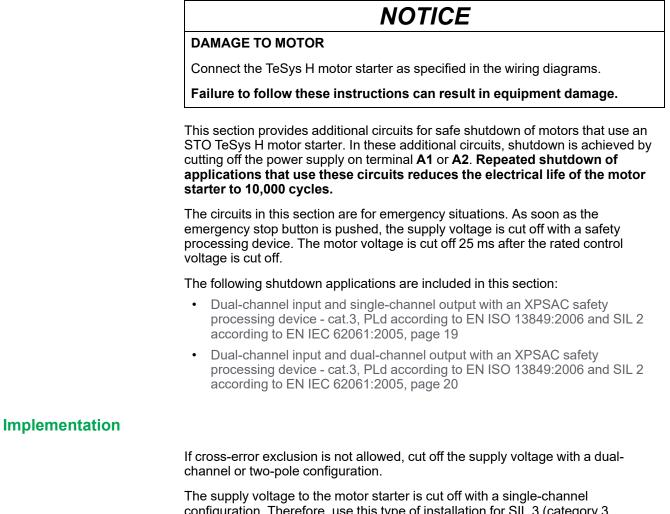
The supply voltage to the motor starter is cut off with a single-channel configuration. Therefore, use this type of installation for SIL 3 (category 3, category 4) **only** if cross-error exclusions are allowed. For example, use this type of installation when the motor starter and the safety processing device are installed in the same control panel.
