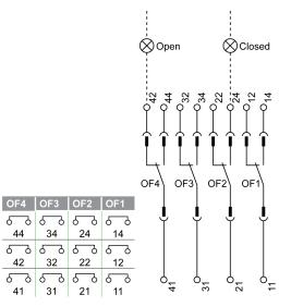
Two additional blocks of four OF indication contacts (OF11–OF14, OF21– OF24) are optional on MasterPact MTZ2/MTZ3 devices.
