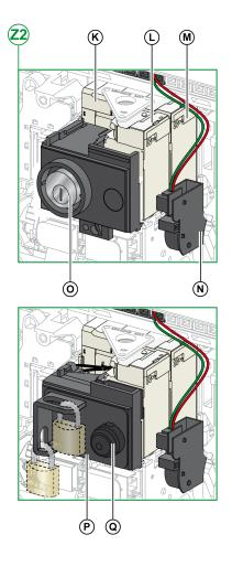
$\boldsymbol{K}$  MN undervoltage release or MX2 opening voltage release
