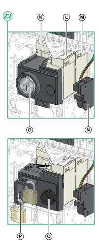
**K** MN undervoltage release or MX2 opening voltage release
