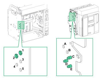
The pin combination selected on the chassis must correspond to the pin combination selected on the device (see following table). For example, the combination 12 on the chassis corresponds to the combination CDE on the device.
