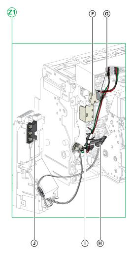
F Standard SDE1 fault-trip indication contact
