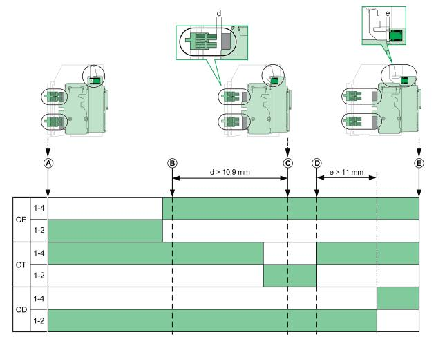
A Device in connected position
