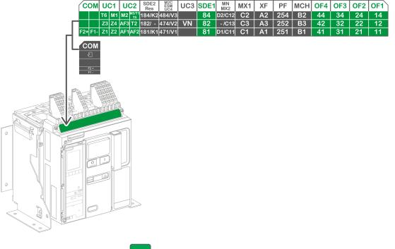
Terminal block supplied as standard on the circuit breaker
