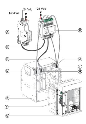
A IFM Modbus-SL interface for one circuit breaker
