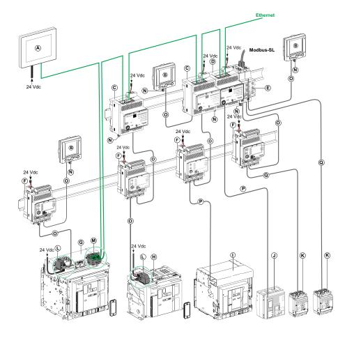
A FDM128 Ethernet display for eight devices
