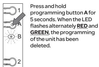
Press and hold programming button **A** for 5 seconds. When the LED flashes alternately **RED** and **GREEN**, the programming of the unit has been deleted.
