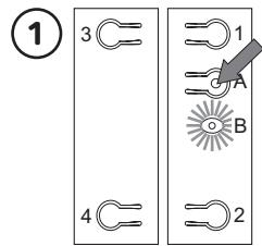
Start the programming by pressing the programming button **A** once.
