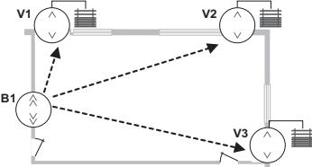
The 3 combined modules for roller blinds **V1, V2, V3**, (receivers) are installed in place of the existing controls. The battery powered push button **B1** (emitter) is used for the centralisation command; it can be fixed onto the wall anywhere. **B1** is associated to **V1, V2, V3** by a Simple link.
