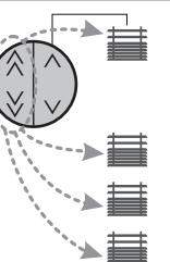
The combined module is both an emitter and a receiver.
