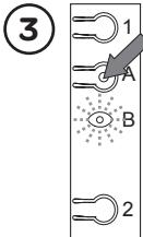
Select the receiver by pressing the programming button **A** once. Wait until LED **B** flashes **RED** (after 5 s with a combined module).
