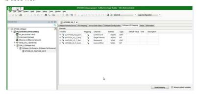
In the PDO Mapping tab, configure and activate the PDOs.
