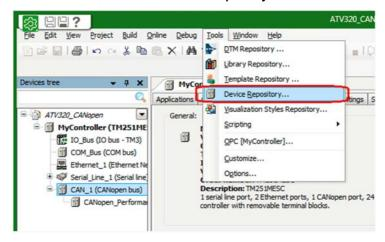
In the Device Repository dialog box, select Remote Device and then click Install.
