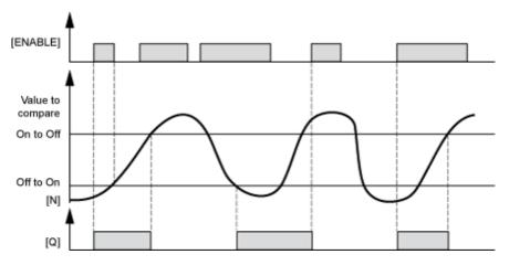
The figure below shows the possible output states when the Off to On setpoint is higher than the On to Off setpoint.
