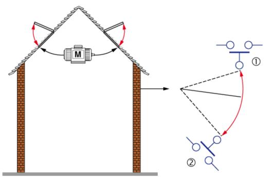
During the day, the panes open to ventilate the structure when the temperature reaches 25°C. If the temperature falls below 20°C, the panes must close again.
