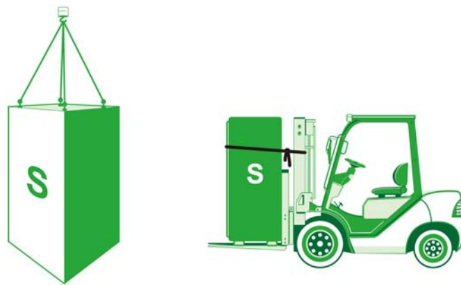
Fig: Lifting and handling
