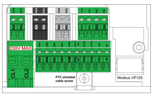
The control terminals are installed with one-way plug-in connectors and can be unplugged during the wiring.
