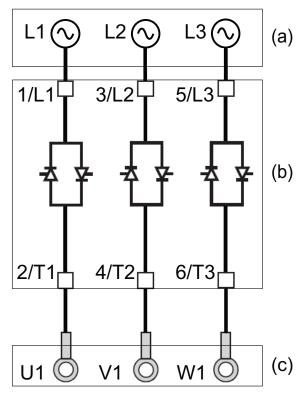
The soft starter can be connected in–line to the motor supply. The motor connection type (star/delta) depends on the supply mains, refer to the motor nameplate.
