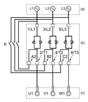
The soft starter can be bypassed with a contactor (K) at end of start. The bypass contactor can be controlled by the soft starter, using the relay R2. The monitoring functions such as current measurement remain active when the soft starter is bypassed.
