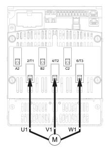
Use class C cables for the power connections.
