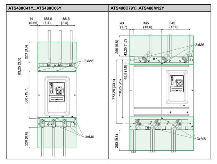
The following measurements are in millimeters (inches).
