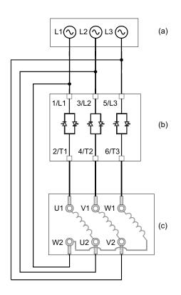
The Soft starter can be connected in series with motor windings in a delta connection (inside the delta connection). By doing so, for the same motor power rating, the current going through the winding and the soft starter is reduced by 1.7 ( $\sqrt{3}$ ). This reduction allows to choose a soft starter with lower current rating.
