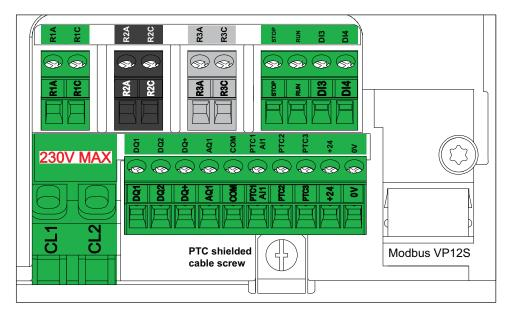
The control terminals are installed with one-way plug-in connectors. Ferrules are mandatory for wiring the CL1 and CL2 terminals to ensure an IP20 protection. The terminals are approved for stranded conductors and solid conductors. Use wire cable ends (ferrules) if possible.
