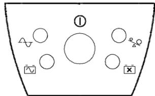
With the UPS plugged in, press and release the on/off/test button to supply power to the loads plugged into the Battery Power Supplied outlets. The equipment plugged into the Full Time Surge Protected outlet (the top outlet) has power whenever the UPS is connected to an active AC power source.
