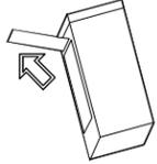
1. Lay the UPS on its left side. Remove the two screws holding on the battery door and open the door.
