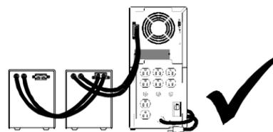
Correctly completed tower XL installation with two battery packs.
