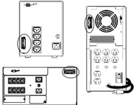
This figure shows the location of the battery pack connector on the SU3000 tower unit (right), the 5U SU3000RM (bottom), and the SU1000XL tower unit (left). Some UPS models have the battery pack connector in different positions, but the size and shape of the connector is always the same.
