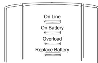
**On Line (green)** - is lit whenever utility power is powering the Battery Backup outlets.
