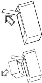
1. Lay the UPS on its left side. Remove the two screws holding on the battery door and open the door.
