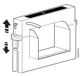
2. Separate the top and bottom sections of the sensor by twisting the sections apart.
