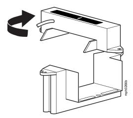
**NOTE:** Make sure the arrow on the Current Sensor is pointing away from the *positive* battery terminal, connected to the lead on which the sensor is placed.
