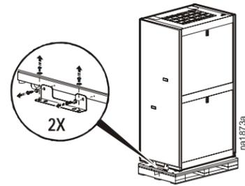
**Note:** If the unit is to be secured to the floor, save the bolts, washers and brackets.
