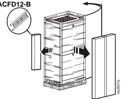
The protective skirt for bottom piped configurations will also be secured with the plastic wrap. Remove this box and set aside.
