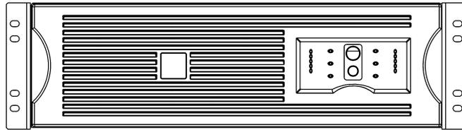
The ON and OFF buttons are used to power the UPS and act as master controls for the connected equipment. (Make sure connected loads are switched to their ON position) The UPS remains on as long as it is attached to utility power.
