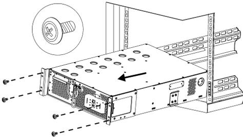
1. Remove the four rack screws (two screws on each mounting bracket) that secure the UPS to the rack.
