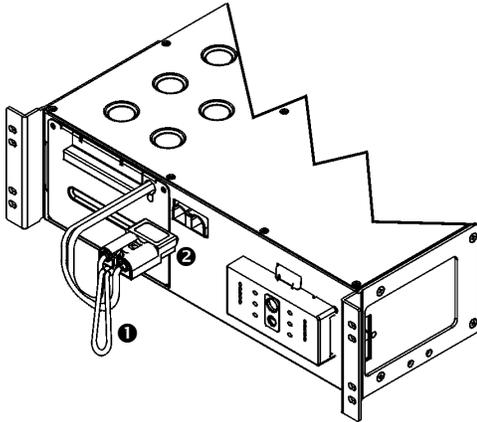
The battery module is accessible from the front of the UPS (shown at left).
