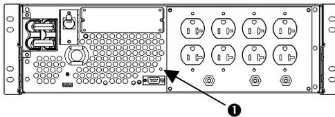
3. **120V Models only:** Connect ground leads to the TVSS screw ❶ on the back panel. The transient voltage surge suppression (TVSS) screw provides grounding through the UPS power cord ground conductor.
