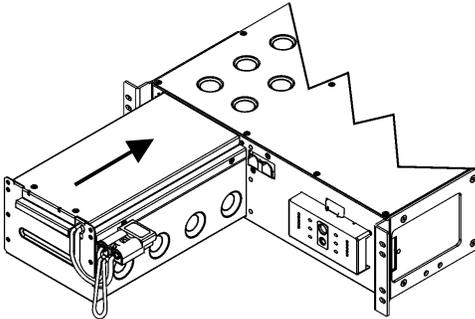
1. Supporting the battery module on the bottom, align it with the opening and slide the battery module into the compartment.
