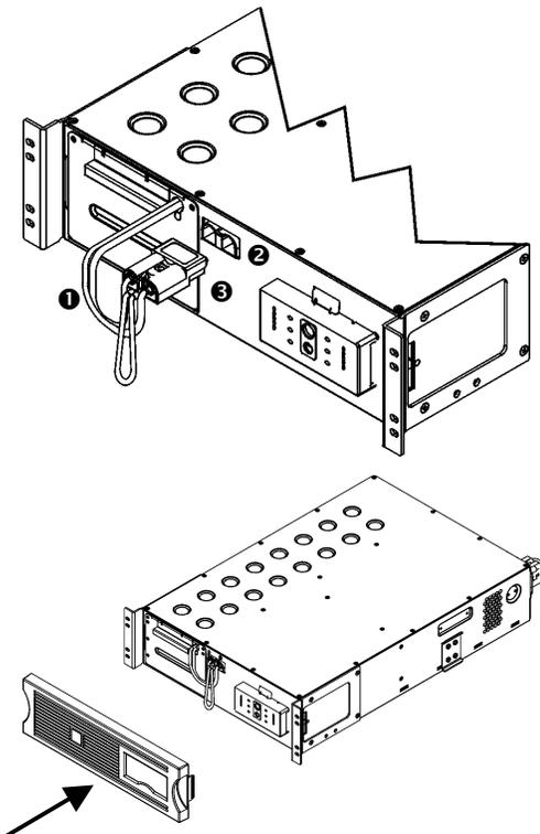
1. Facing the front of the UPS, locate the battery cables ❶ and the UPS battery connector jack ❷ to the right of the battery module.
