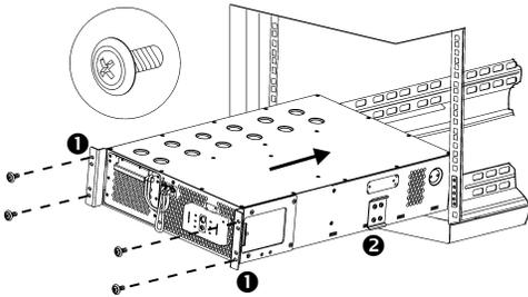
1. Supporting the UPS on both sides, carefully align the unit with the rails. Use the handles 1 on the side of the UPS to support the unit.
