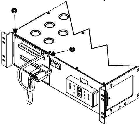
2. Use a screwdriver to remove the two battery module mount screws located at the top corners of the face plate **3**.
