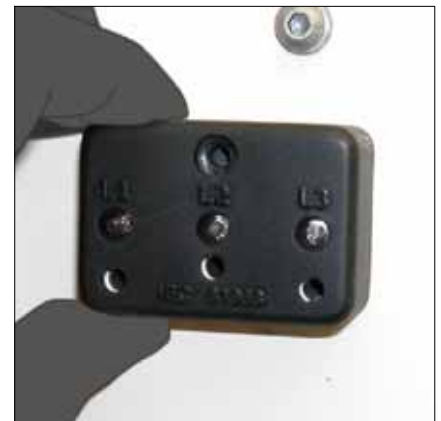
J Connect a new unit. J Lightly tighten the fixing screw.
