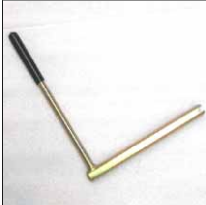
J Standard operating lever for the load-break switch (black end).
