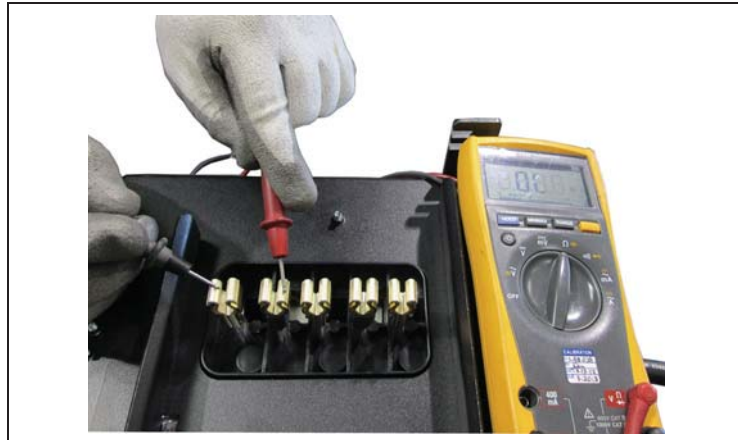
Figure 5: Testing for Plug-In Unit Isolation Prior to Installation
