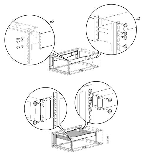
The UPS mounting rails provide room to mount additional equipment behind the UPS (fasteners for equipment mounting not included).
