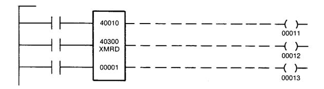
In this example, a block of 1400 6XXXX registers are read in two scans (700 per scan) from extended memory. The block starts at register 3000 in file three and is written to a block starting at register 40300.
