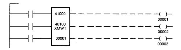
In this example, a block of 1000 4XXXX registers is written in one scan to extended memory. The block starts at register 41000 and is written to a block starting at register 2000 in file two.
