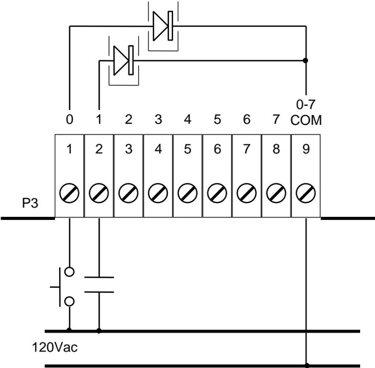
Figure 2: AC Input Wiring Example
