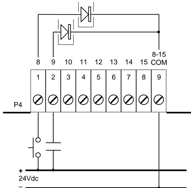
**Figure 3: DC Input Wiring Example**
