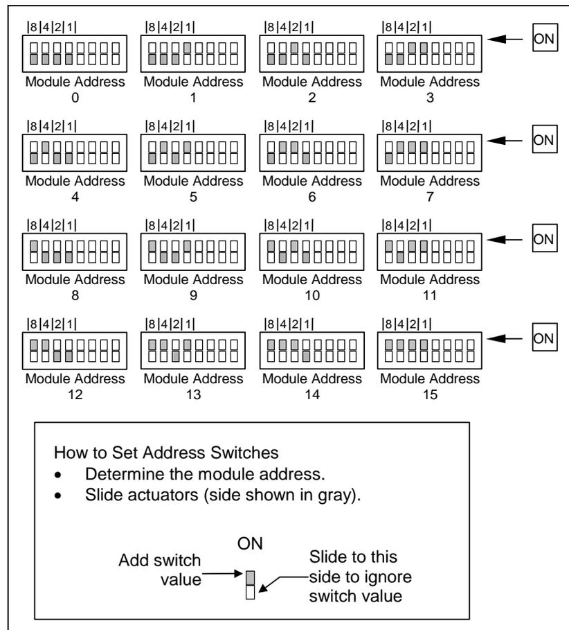
**Figure 4: 5405 Digital Input Module Address Switches**
