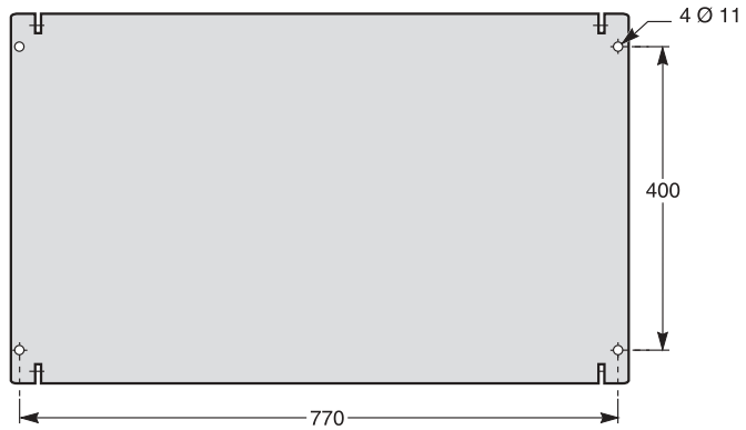
Fig. 9 bis: plinth for cubicles A2, A3, cat. no. 52673.
