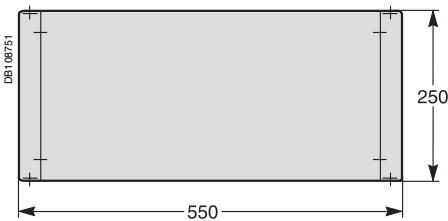
Fig. 8: freestanding plinth for enclosures, cat. no. 52671.
