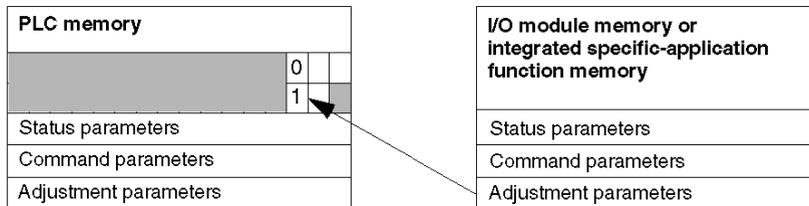
When the data is exchanged between the PLC memory and the module, acknowledgement by the module is managed by the `ADJ_ERR` bit (`%MWr.m.c.1.2`).
