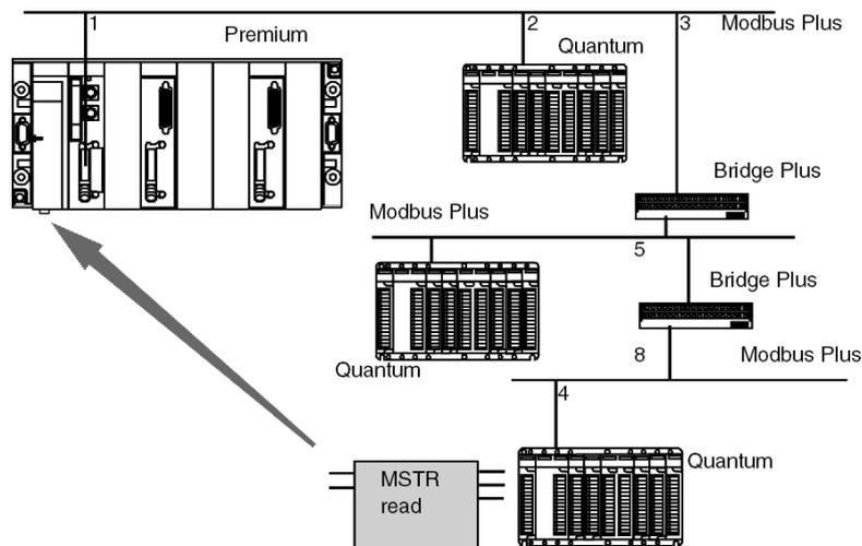
The Quantum station sends a read request to the Premium station using the following address path: 8.5.1.0.0 (routing path).
