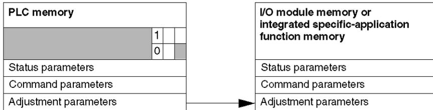
When the instruction is scanned by the PLC, the **Exchange in progress** bit is set to 1 in `%MWr.m.c`.
