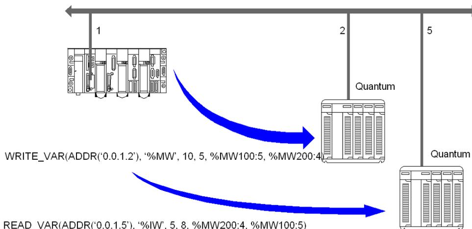
The internal words to write to station 2 are located at address 10.
