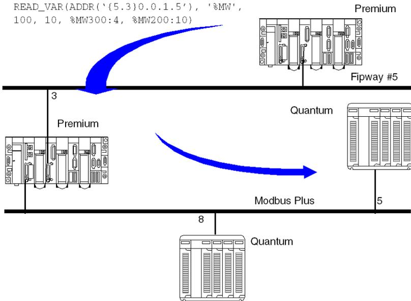
**NOTE:** The routing between Fipway and Modbus Plus is performed automatically by the system. In a network architecture, it is not necessary to declare a bridge station.
