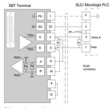
Rt line impedance matching resistor
