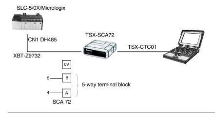
How to Connect a PC in Multidrop Mode to a DH485 Network
