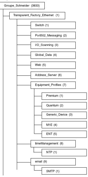
The **Groupe\_Schneider (3833)** subtree is the root of Groupe Schneider's private MIB in the Structure of Management Information (SMI) used by SNMP and defined in RFC-1155, which is a specification that defines the structure and identification of management information for TCP/IP-based networks.
