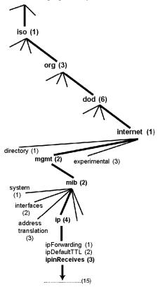
This object name is represented in an SNMP message by assigning each part an integer. So, the above message would appear as 1.3.6.1.2.2.4.3.
