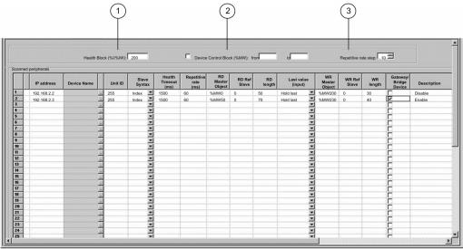
**NOTE:** This screen shows I/O Scanner services for an 140 NOE 771 01 or -11 module. The **I/O Scanner** screen is slightly different for the CPU 651 x0 module, which does not display a **Health Block** field.
