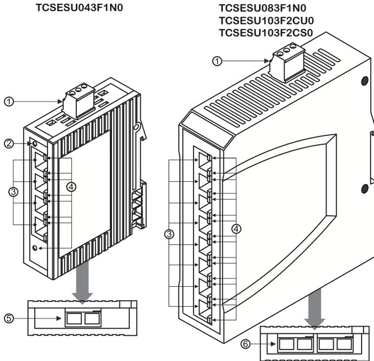
**NOTE:** Remove the rubber cover on the bottom of the switch to access the fiber-optic ports.
