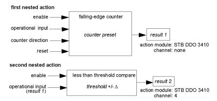
Result 2 (from the compare block) is the result that the nested reflex action will send to an actual output. Because the result of a compare block needs to be mapped to a digital action module, result 2 is mapped to channel 4 on an STB DDO 3410 digital output module.
