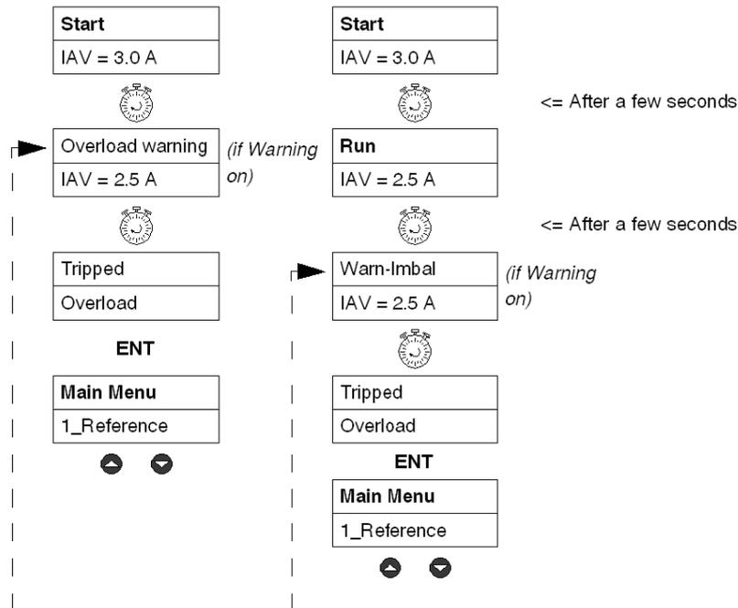
Returns to current mode if no key is pressed for 30 seconds.
