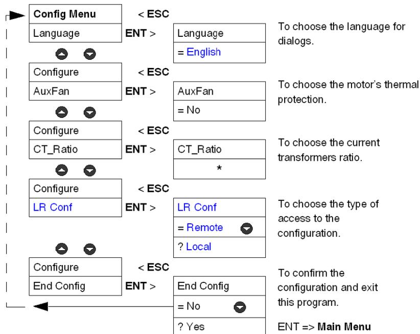
\* No transformation ratio is saved in the factory settings. This parameter must be entered before you can exit the **Config Menu** program.
