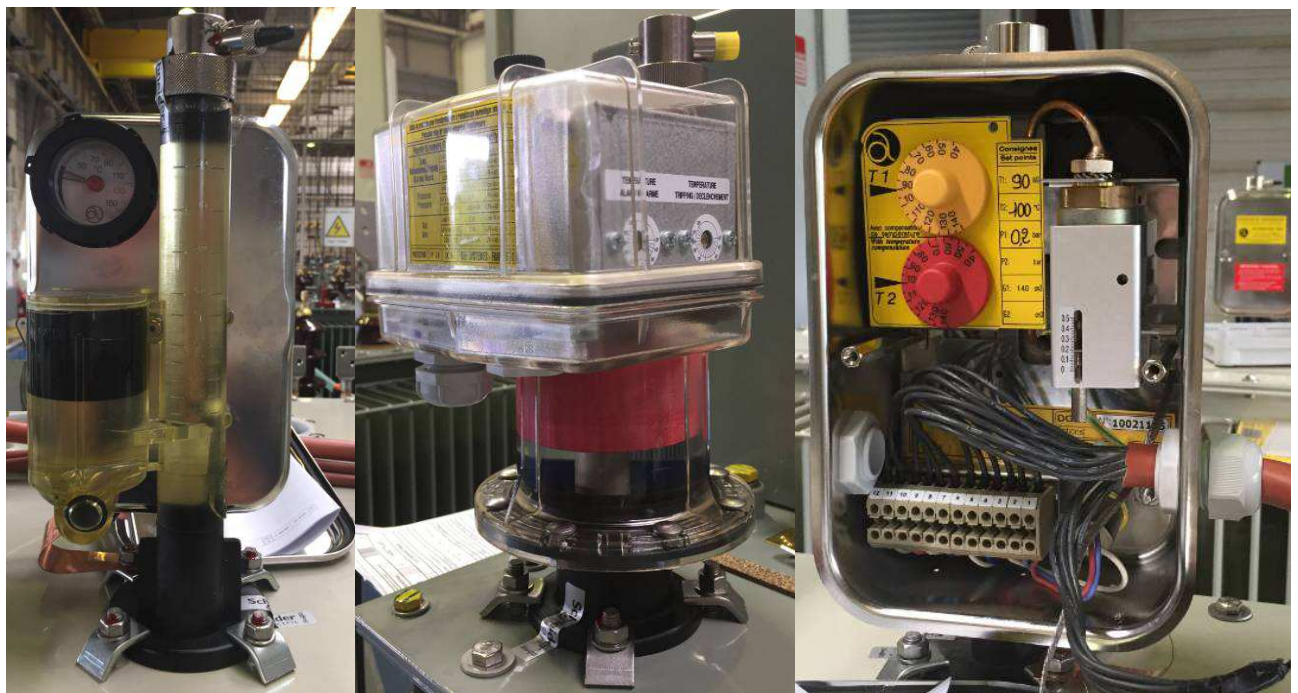
Fig. 15. Views from the left: DGPT2 seen from the oil level protection side, DMCR - general appearance, DGPT2 inside view during wiring.
