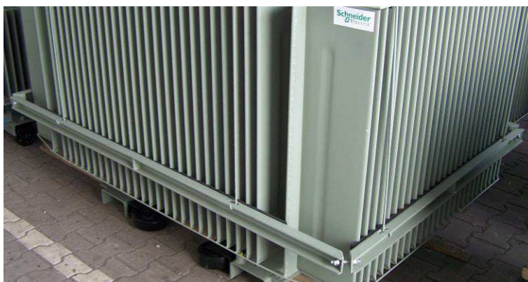
Fig. 20 Protection system with beams for transport purposes.
