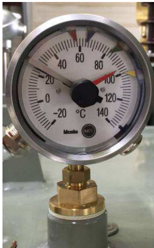
Fig. 12. Typical appearance of a thermometer placed in a thermometer pocket.
