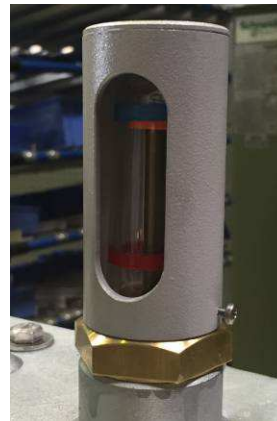
Fig. 10. . The floater head in the minimum position. Operation of the transformer below that position is forbidden.
