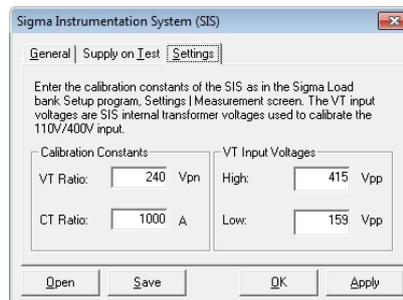
The Values shown above are the default values as normally set up as factory defaults in the SIS.
