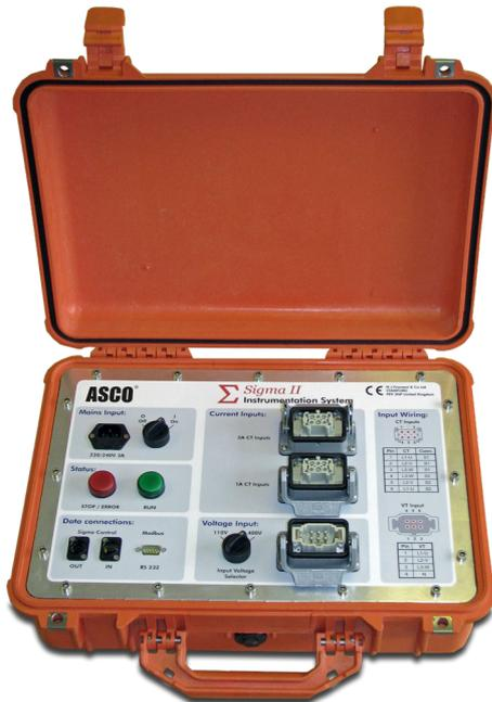
The SIGMA Instrumentation System (SIS) is used, in conjunction with the SIGMA PC program, to display and capture the three phase instrumentation directly at the Supply on Test. When a SIGMA controlled load bank and SIS are used together on the SIGMA 'network' the SIGMA PC System will also enable load control at the load bank.
