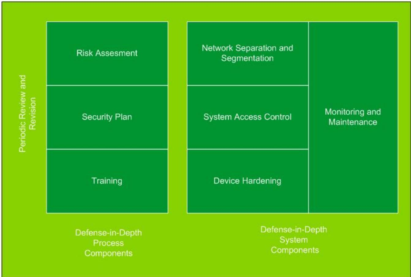
**Figure 13: EcoStruxure Plant Network Defense-in-Depth Components**
