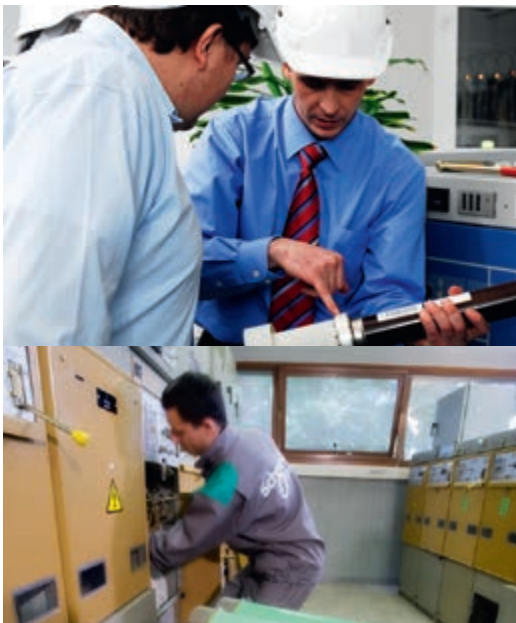
OnSite ProDiag Fuse diagnoses the condition on de-energized medium voltage fuse component
