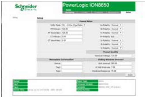
Example embedded webserver page (WebMeter) showing realtime values.
