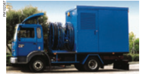
Clipper M on truck with cable roller
