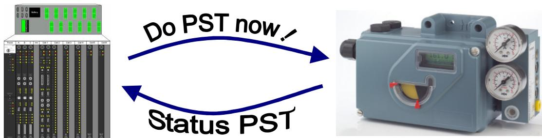
The communication protocol is used only to send information to a PC or a DCS in charge of the diagnostic and predictive maintenance.
