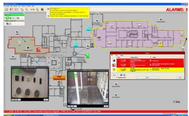
Esgraf 4.1 brings fire detectors contamination information in to our graphical user interface. Contamination information from fire detectors can be read and saved in to Esmikko4 database server e.g. once a day, from where Esgraf can read and show it graphically.
