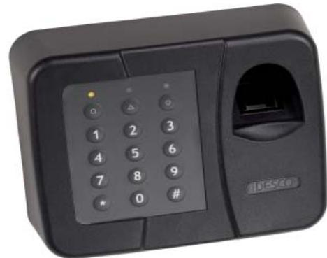
Access MFinger is a high security biometric reader combining security features of the Mifare® smart card technology and the user's individual and unique fingerprint. The reader compares a fingerprint stored into a Mifare® smart card with the scanned fingerprint before transmitting data into the system. Mifare® security keys protect the templates inside the card. It is also possible to store fingerprint templates into the Access MFinger reader.
