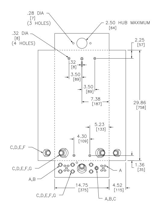
FINISH - GRAY BAKED ENAMEL ELECTRODEPOSITED OVER CLEANED PHOSPHATIZED STEEL.
