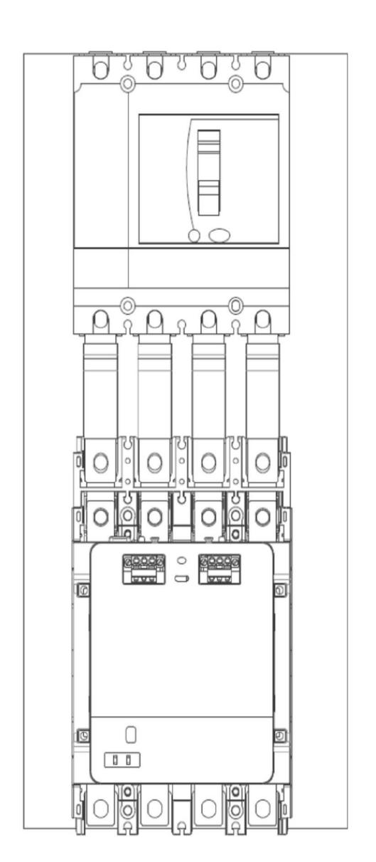
Installation Note NSX100-250 - Flexible bar - Cable memory - LC1G115-225 4P
