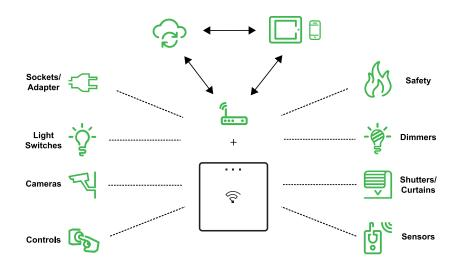
The Wiser gateway is the center of the system, processing control requests and status reports for connected Wiser devices.
