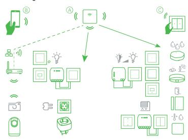
The Wiser gateway (see A) is the center of the system, processing control requests and status reports for connected Wiser devices.
