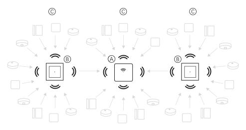
**TIP:** Install and commission all mains-powered devices before commissioning battery-powered devices. This provides maximum hosting capacity prior to adding the battery-powered devices.
