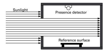
Optimal light conditions for actual value correction. Measurement results at the installation site or at the reference area are affected equally by natural light.
