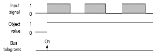
3. Configured with edge evaluation: "falling On "
