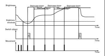
The movement detector changes to non-brightness-dependent mode once the start of movement action (sending an ON telegram) has been carried out. Here freshly detected movements can retrigger the staircase timer. The movement detector cannot process the brightness jump and there is not even any setting of a hysteresis.
