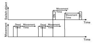
In master mode or normal mode the movement time corresponds to the staircase timer in the diagram above. In slave mode or monitoring mode the movement time corresponds to the cycle time. In practice a large number of applications can be implemented by means of the various blocks.
