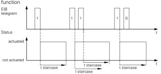
Retriggerable staircase lighting function without manual OFF function
