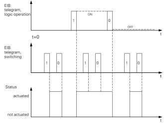
The relay can only be opened via the "Switch object" once a "0" telegram has been received via the "Logic object".
