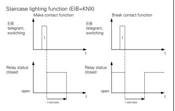
The period (t staircase) is calculated by multiplying a base value by a factor.
