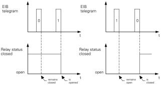
After bus voltage recovery, the relay is closed in the "break contact" mode and a status response telegram is generated with the value "1" if the status response function is activated. In this case, a different response is carried out e.g. by a higher priority function or due to the behaviour on bus voltage recovery at the output.
