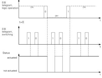
The logic object is preassigned the value "1" after a RESET. The actuator will immediately switch on the output in the "make contact" mode. The OR logic function is only reset by a "0" telegram at the logic object.
