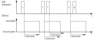
For the staircase lighting function, you can use the parameter "with / without manual OFF function" to set whether the timer is switched off prematurely after a
