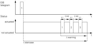
In the case of staircase lighting functions with a manual OFF function and active prewarning, the staircase lighting function with prewarning is immediately deactivated when an OFF telegram is received.
