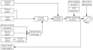
With regard to the switching behaviour of the actuator, each function has a certain priority. The weighting of the functions can be taken from the following table:
