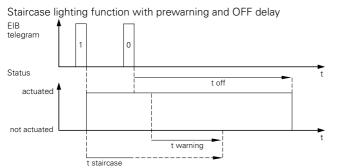
In the case of staircase lighting functions with a manual OFF function and active prewarning, the staircase lighting function with prewarning is immediately deactivated on receipt of an OFF telegram. The OFF delay elapses. No prewarning takes place.
