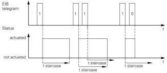
The staircase lighting function can indicate that the end of the staircase timer is imminent by causing the luminaire to flicker. It is possible to select between one and three warnings. It is possible to set the time (t warning) when the warnings should start before the staircase timer has elapsed. The length of the interruptions (t I) and the interval between two warnings (t int) can also be set.
